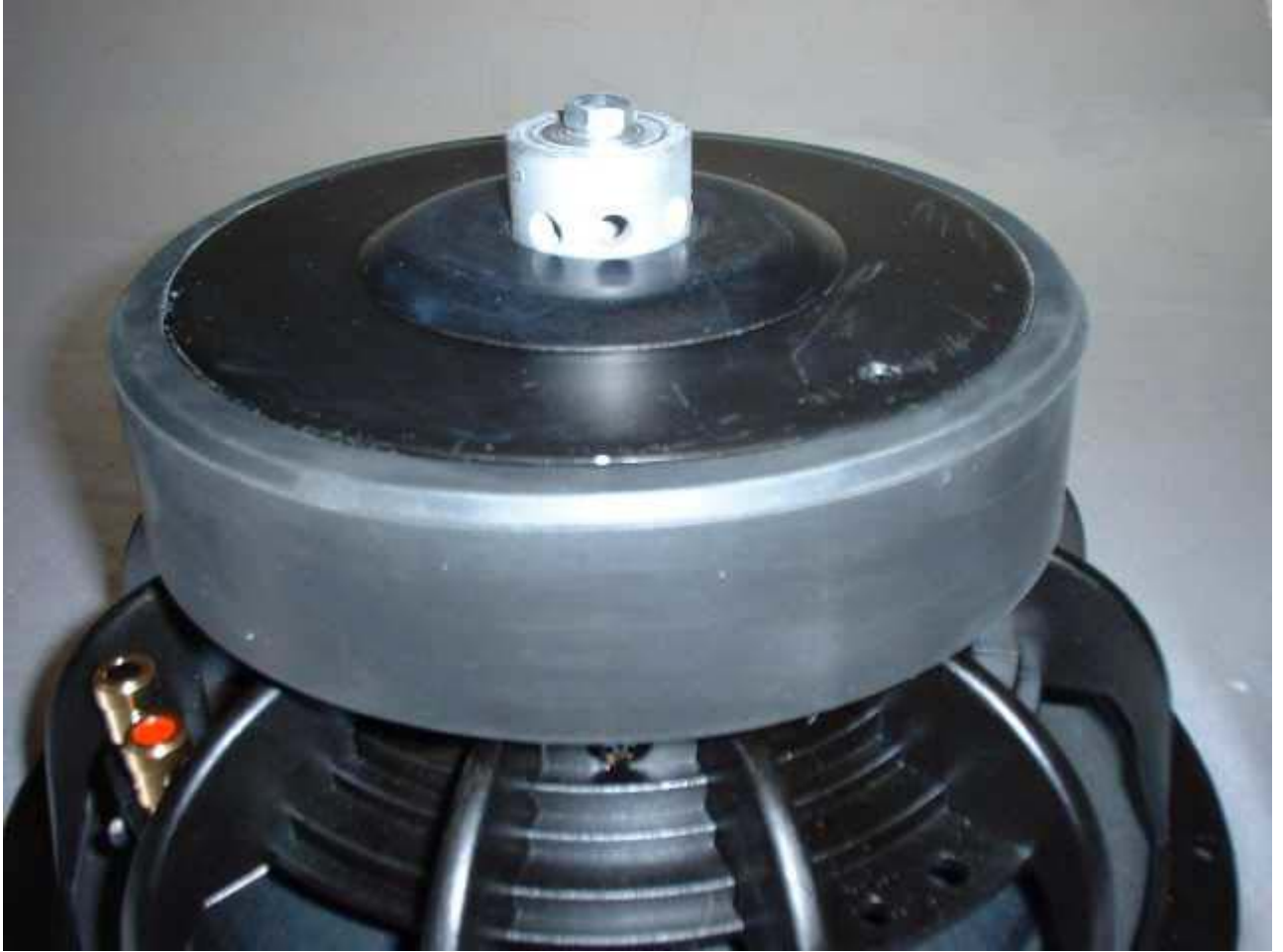
Cooling plug inserted, ready to attach to the heat exchanger
