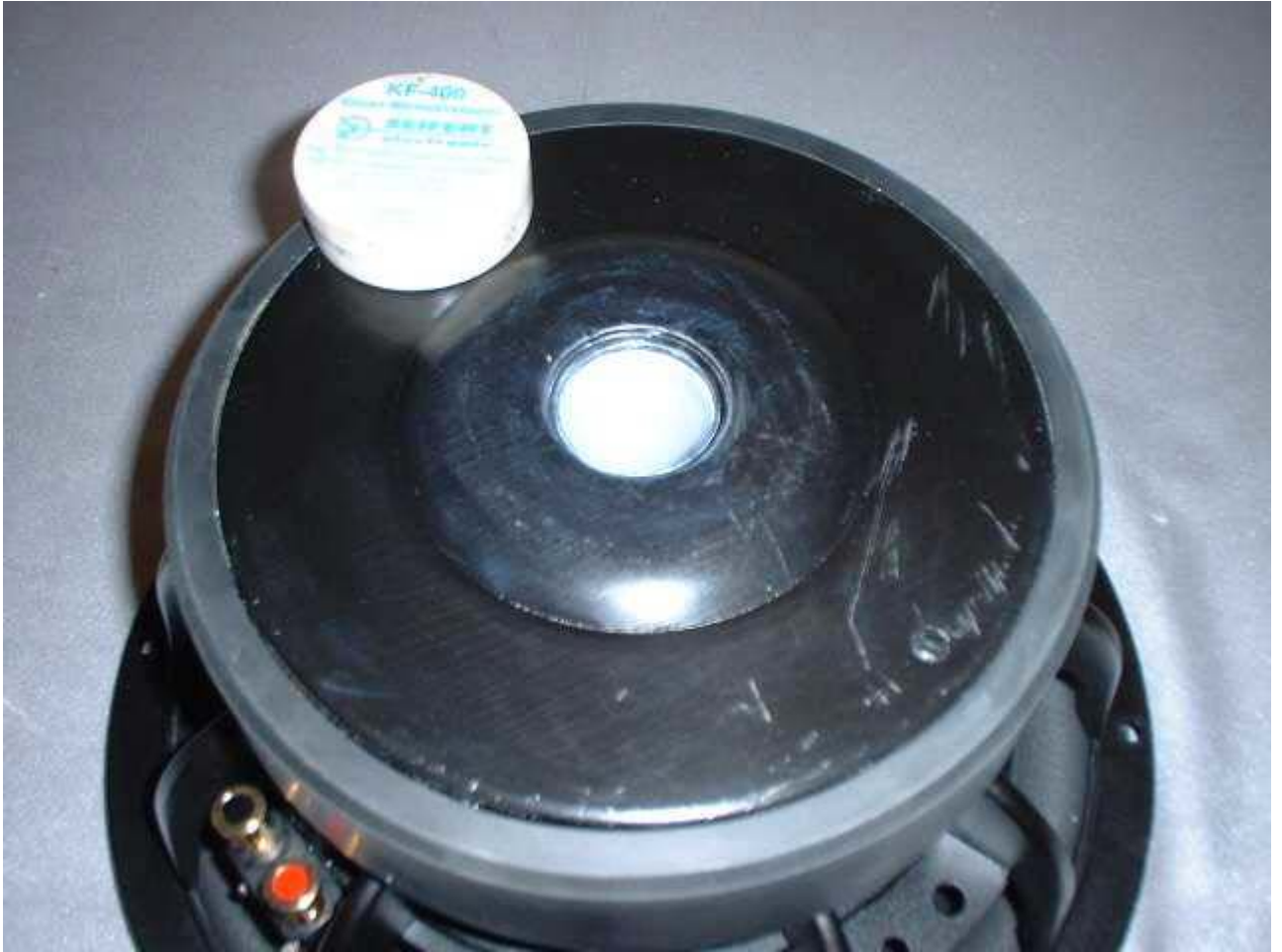
Heat conductive grease on pole piece, in vent hole
