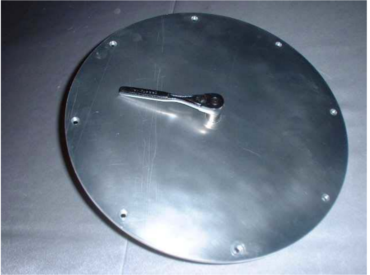
Fastening the plate to the cooling plug
