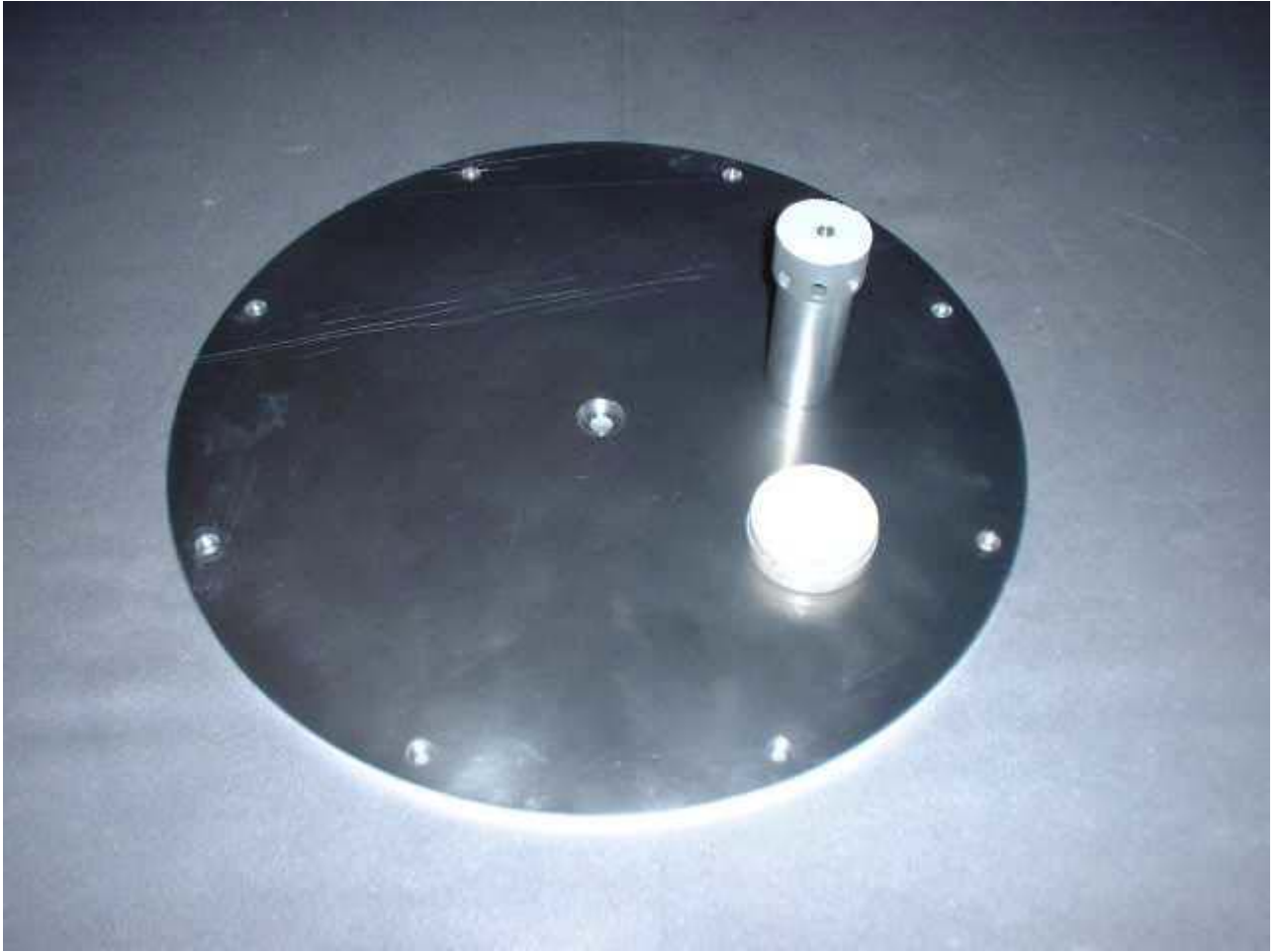
Heat conductive grease applied to cooling plug prior to attaching heat exchanger plate
